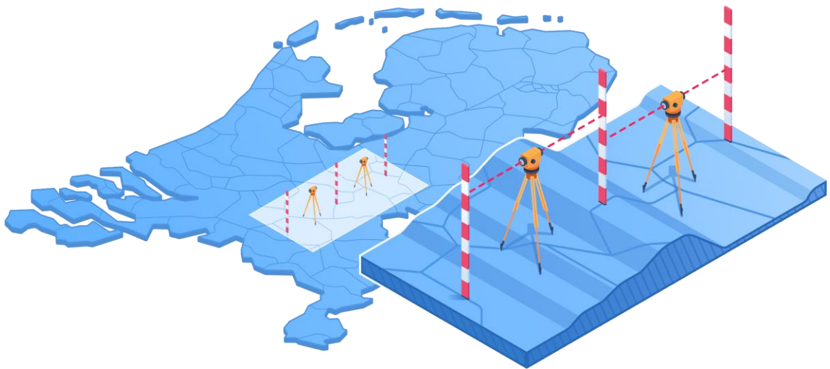
Figure 83. Levelling for establishing the NAP
