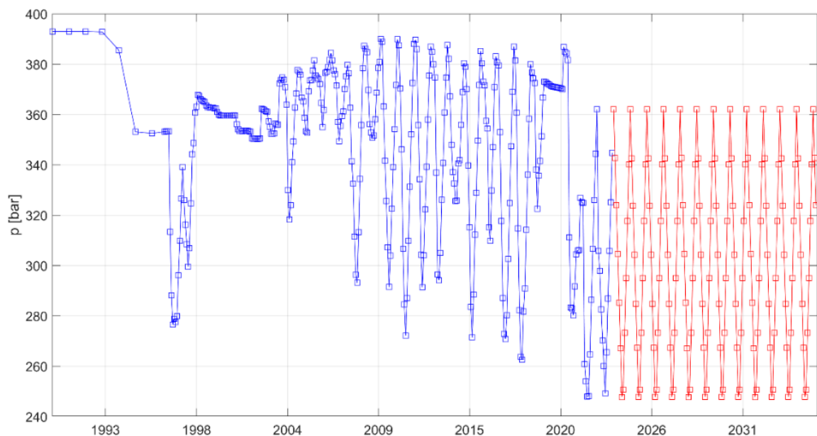
Figure 50: Temporal evolution of the pressure in the Grijpskerk reservoir. The reservoir was turned into an underground gas storage facility (UGS) in 1997. Prior to 1997, gas has been produced from the reservoir, reducing the reservoir pressure to 353 bar. Future pressure evolution (after end 2023, red curve) is “forecasted” by extrapolating the pattern of the years 2021/2022/2023.
