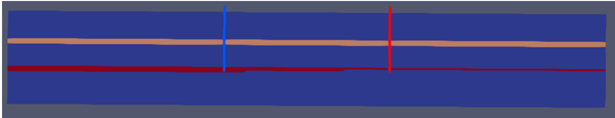
Figure 4-13: Cross-section of numerical model for the stepwise thickness variation case. Bottom reservoir thickness at the producer well equal to 16.7 m (case h2).
